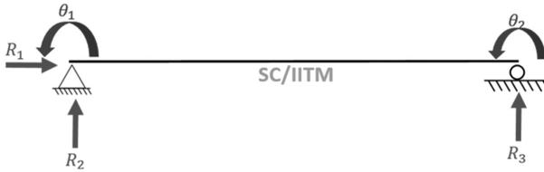
FIGURE 1.3 Simply supported beam.
